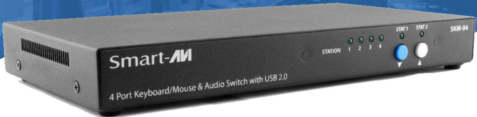
Manage Keyboard and Mouse operations on four computers from a single workstation with support for USB 2.0 sharing
