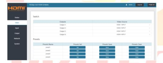
To this preset setting, first you need to select the desired input source to four output ports. Then click the Save button to save the setting. When you click the line Set button, this preset you have saved will be used. The Clear button will clear the preset. There are four presets setting available.
