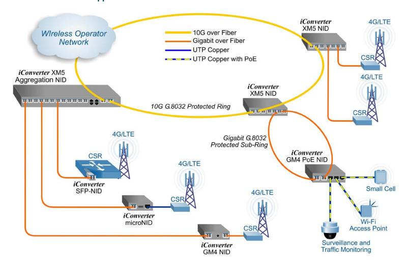
In this Carrier Ethernet mobile network application, iConverter Network Interface Devices (NIDs) are deployed throughout Ethernet Mobile Backhaul and Radio Access Networks (RAN).
