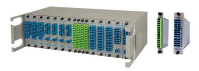
OmniLight CWDM and DWDM modules expand fiber capacity with up to 24 channels, and up to 10G per channel. They support legacy 1310, 1550 pass band ports, and OTDR port for fiber troubleshooting and testing. The passive optical modules support dual fiber duplex and/or single-fber simplex (BIDI) with an optional cascade port for future capacity expansion, and unidirectional/bidirectional monitoring ports for diagnostics and testing.
