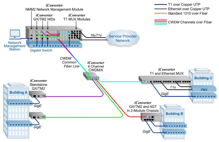
In this campus network application diagram, the iConverter Multi-Service Platform enables multiple services to be transported over CWDM with connectivity to copper equipment in different buildings.
