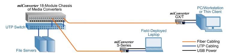
In this application diagram, miConverter media converters enable cost-effective fiber-to-the-desktop connectivity that is reliable and easy to install.
