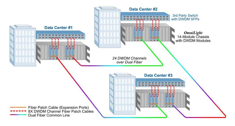
Data Centers often have a cluster of Storage Area Networks (SAN) servers and storage discs connected using Fibre Channel or Ethernet. Data Centers require high speed connectivity to off-site locations for database mirroring and replication. To provide redundancy and disaster recovery, a SAN in one Data Center can be extended to a SAN in another Data Center. This allows each Data Center to have a mirror copy of its data at each location.
