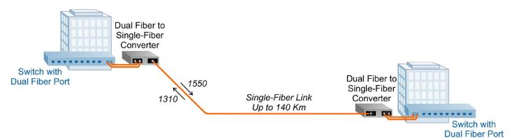
Networks may require conversion between dual and single-fiber, depending on the type of equipment and the fiber installed in the facility. Single-fiber is single-mode and operates with bi-directional wavelengths, often referred to as BIDI. Typically BIDI single-fiber uses 1310nm and 1550nm wavelengths over the same fiber strand in opposite directions.
