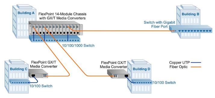
In this application example, FlexPoint GX/T media converters are deployed in a star topology network with multiple fiber links distributed from a central location. At Building A, a FlexPoint 14-Module Chassis with GX/T media converters are used to convert the RJ-45 ports from the copper switch to fiber links.
