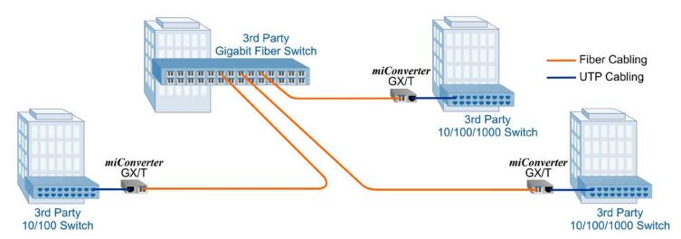
In this application diagram, miConverter media converters enable campus network fiber connectivity to existing copper network switches.
