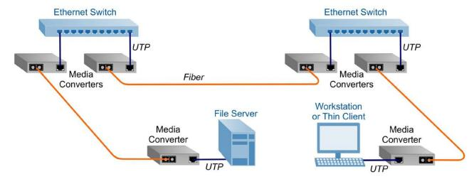
This application example demonstrates how copper to fiber media converters enable fiber connectivity to extend network distances. FlexPoint copper-to-fiber media converters support a variety of cabling and connectors, different network protocols, and data rates from 10 Mbps to 1 Gigabit.
