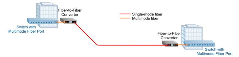
Networks often require conversion from multimode (MM) to single-mode (SM) fiber, which supports longer distances than MM fiber. Fiber-to-fiber media converters can extend a MM network across SM fiber with distances up to 140km for Fast Ethernet (100Mbps) and 80km for Gigabit Ethernet (1000Mbps) and 10 Gigabit.
