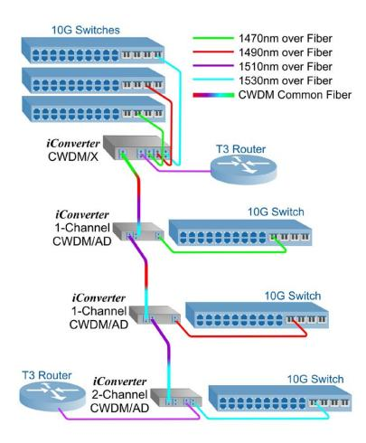
In this application diagram, four CWDM data channels (wavelengths 1470, 1490, 1590 and 1610) are multiplexed onto a CWDM Common Fiber Line, and the wavelengths are dropped off at different locations.
