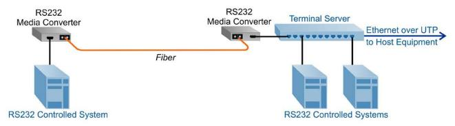
In this industrial/manufacturing network application example, two RS-232 media converters provide fiber distance extension from a Terminal Server to a remote RS-232 controller.
