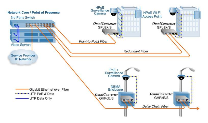
In this application example, Wi-Fi services and security surveillance are delivered over a fiber network with extended distances between network devices. This application shows a campus or municipal fiber network, but these devices can be deployed in a similar fashion at an airport, retail shopping mall, sports arena or any facility with distances that require fiber network connectivity.
