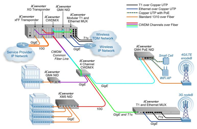
In this application diagram, the iConverter Multi-Service Platform enables multiple services to be transported over a CWDM fiber access network.
