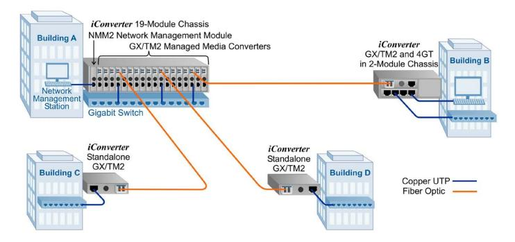
This application example illustrates how the iConverter Multi-Service Platform enables the delivery of gigabit Ethernet in a managed campus fiber network.
